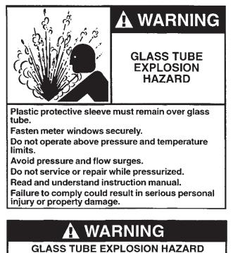
Protective sleeve must remain over glass tube. Fasten meter windows securely. Failure to comply could result in serious personal injury or property damage.
